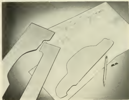
2. From your drawings—or clay model—draw and cut out of cardboard an accurate side view pattern of your model.
